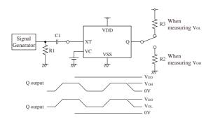
XT input signal: 2.5Vp-p, 10MHz, sine wave C1 = 0.001 $\mu$ F, R1 = 50 $\Omega$ , R2 = 417 $\Omega$ , R3 = 434 $\Omega$ , V<sub>C</sub> = 1.65V
